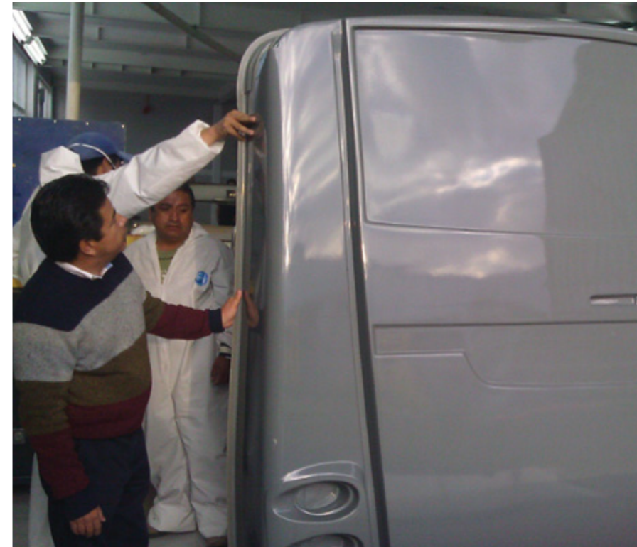
First L-RTM rear mask after demolding
