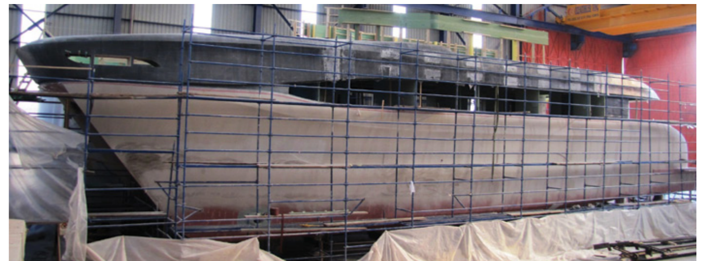
Carbon reinforced epoxy hull structure
